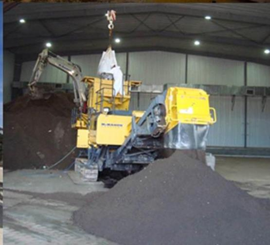
*RemBind®* (US Patent 8,940,958), a powdered reagent manufactured by Ziltek Pty Ltd that binds up and immobilizes contaminants in soil. *RemBind®* is typically added at less than 5% by weight using conventional soil blending equipment. Binding occurs within 24hrs.
