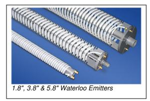
The patented technology (U.S. Patent # 5,605,634) enables steady, direct diffusion of oxygen into an aquifer through pressurized silicone or LDPE tubing. Continuous, consistent release of oxygen into the tubing creates the ideal concentration gradient driving this passive system, without 'bubbling off' excess oxygen.
