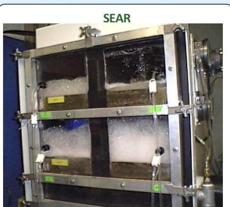
Foam issue experiments on membrane processes for SEAR such as surfactant ultrafiltration for surfactant recycling and air stripping for volatile organic compound removal in waste streams
